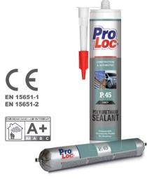
One-component, high-modulus polyurethane sealant that cures on exposure to atmospheric humidity. It possesses excellent adhesion to sheet iron, aluminum, stainless steel, lead, copper, ceramic, glass, wood and various plastic materials.
