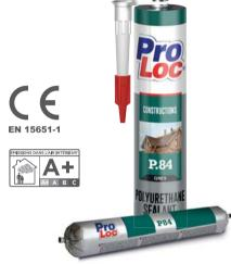
One-component, high-modulus polyurethane sealant that cures on exposure to atmospheric humidity. It possesses excellent adhesion to sheet iron, aluminum, stanless steel, lead, copper, ceramic, wood etc.
