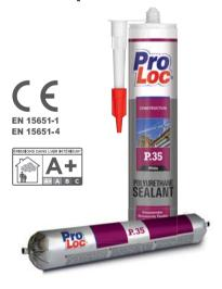
One-component, low-modulus polyurethane sealant that cures on exposure to atmospheric humidity. It possesses excellent adhesion to all typical construction materials such as cement based materials, brick, ceramic, glass, wood, galvanized and painted sheet iron and various plastics.
